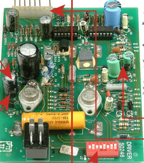
We replace and upgrade all defective low-temperature, low-quality electrolytic capacitors to 105°C. Upgrading from 85°C to 105°C more than doubles the life of your capacitors.
